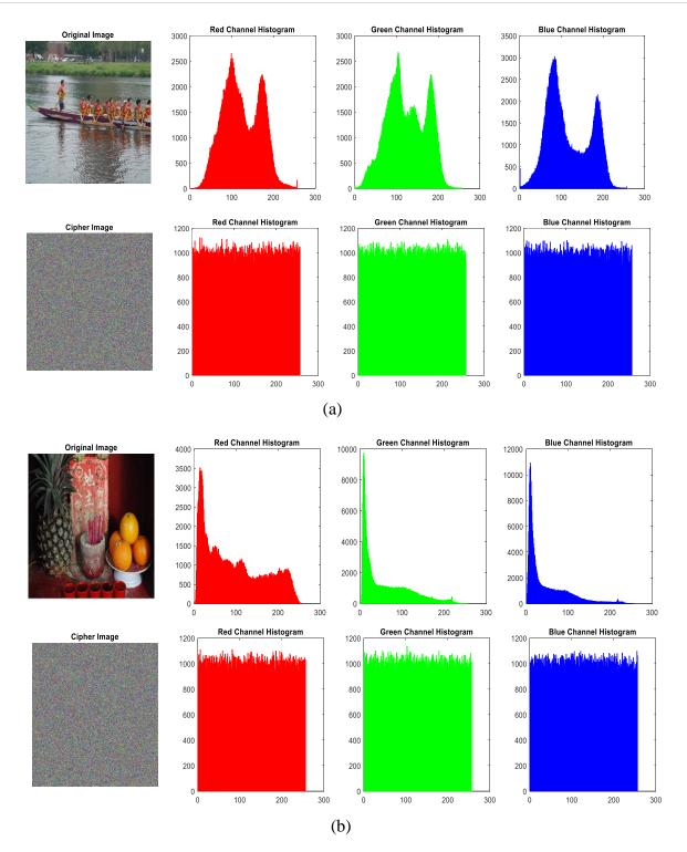
Figure 6: Histogram analysis of original images (a) and (b) with their cipher images according to R, G, B color.
