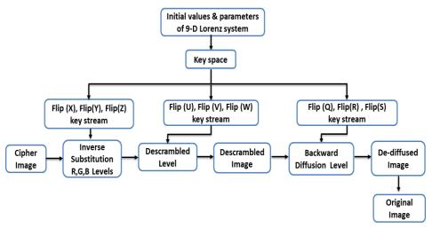
Figure 2: Framework of decryption algorithm
