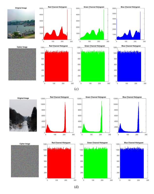
Figure 7: Histogram analysis of original images (c) and (d) with their cipher images according to R, G, B color.
