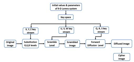
Figure 1: Framework of encryption algorithm.
