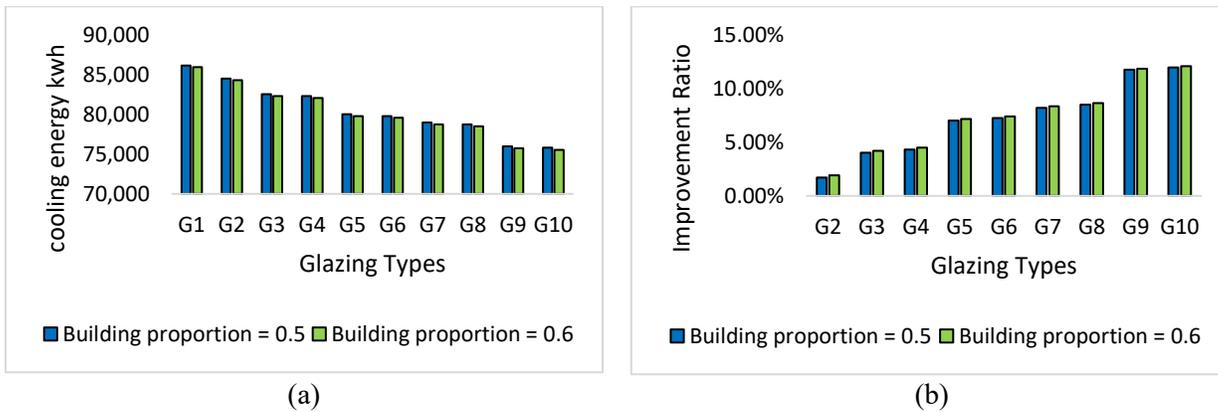
**Figure 4:** Simulation results for building proportion 0.5 & 0.6 considering different glazing types; (a) annual energy saving, (b) improvement rate (%) in terms of energy savings.
