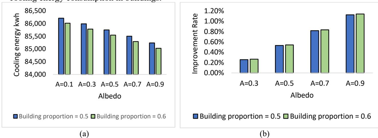
**Figure 5:** Simulation results for building proportion 0.5 & 0.6 considering roof surface albedo; (a) annual energy saving, (b) improvement rate (%) in terms of energy savings.
