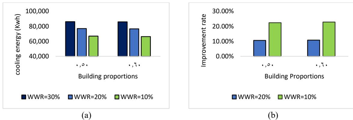
**Figure 3:** Simulation results for building proportion 0.5 & 0.6 considering different WWRs; (a) annual energy saving, (b) improvement rate (%) in terms of energy savings.
