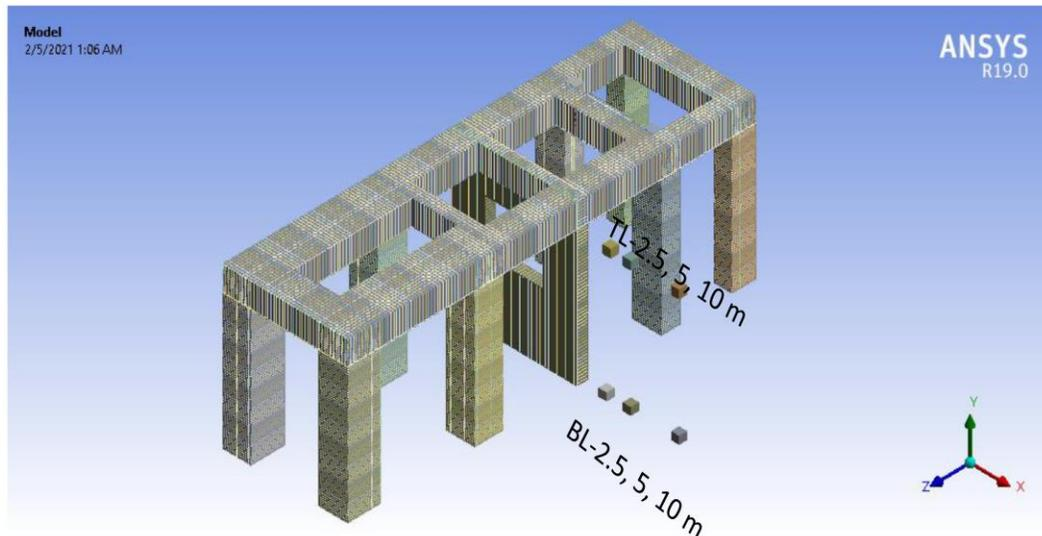
Fig. 4 Top/Bottom Location of TNT at the Short Direction of the Frame
