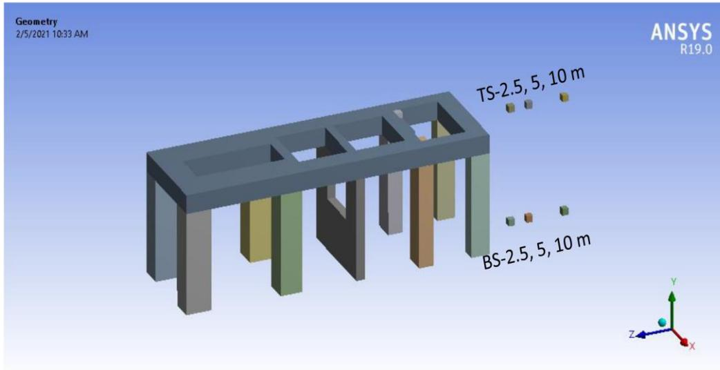
Figure (3) T Figure (4) Top/Bottom Location of TNT at the Long Direction of the Frame
