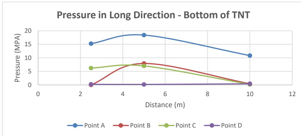
Figure (7) Pressure in Long Direction Bottom of TNT
