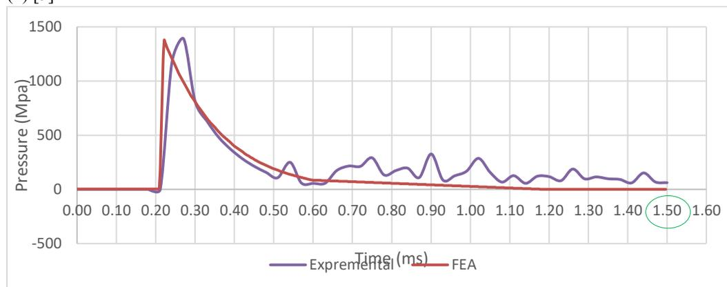
Figure (2) Verification of Blast Pressure.
